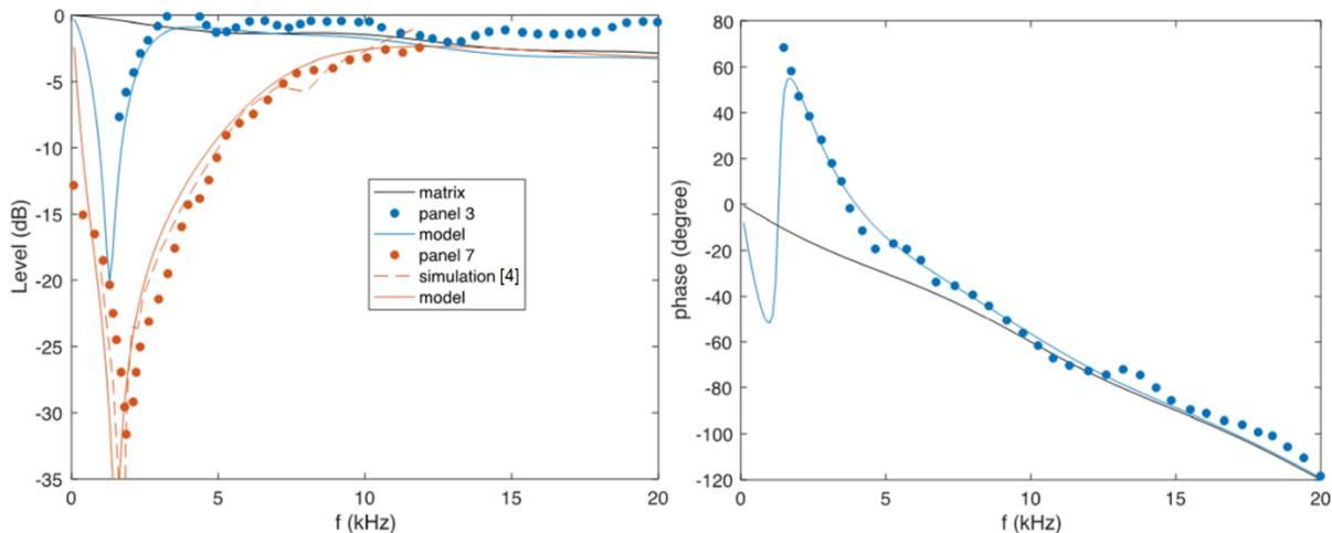
Figure 5: Results for tests panels n°3 and 7, with periodic distribution of voids and silicone matrix
