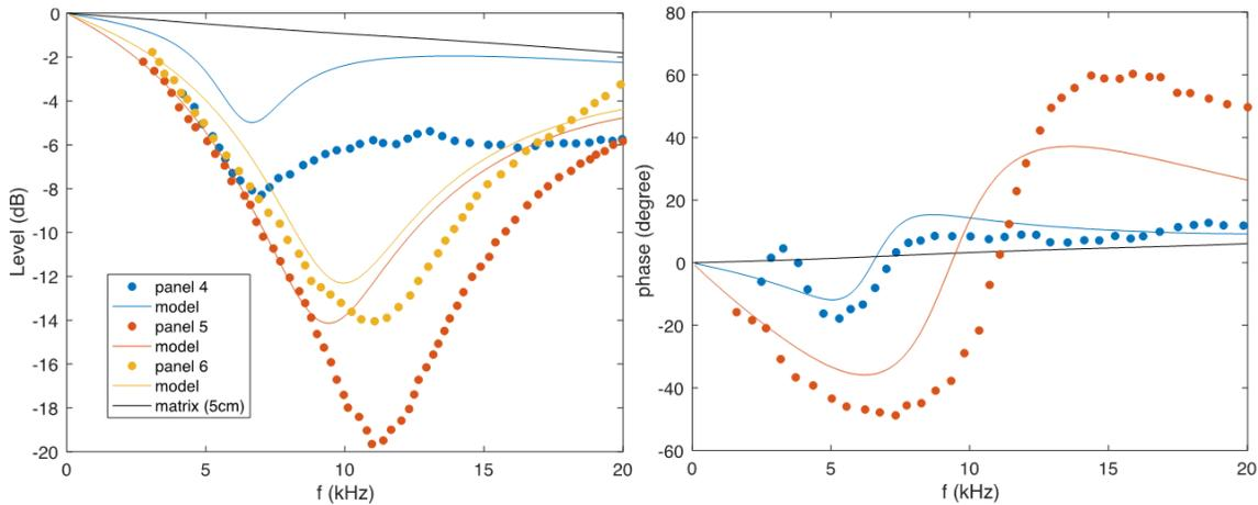
Figure 4: Results for tests panels n°4-6, with periodic distribution of voids and polyurethane matrix
