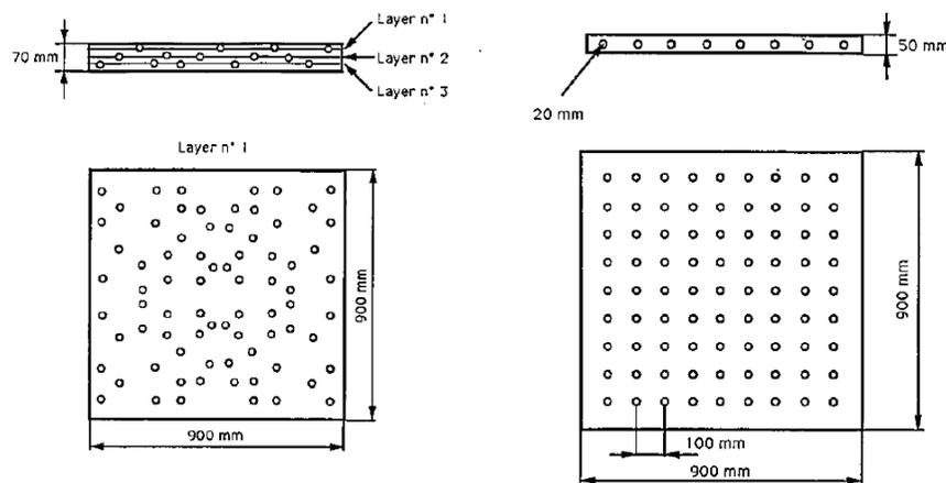
Figure 2: Internal structure of test panels N°1 (left), and N°3 (right), from [5].
