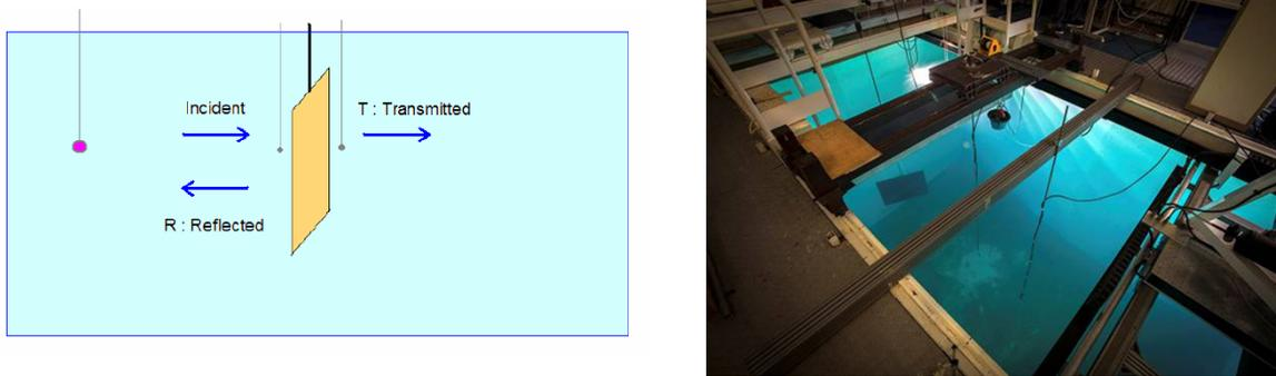
Figure 3: Principle of the acoustic measurement of a test panel and example of water tank facility
