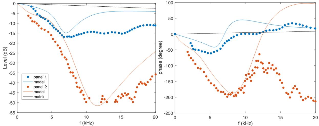
Figure 6: Results for tests panels N°1 and 2, with random distribution of voids and polyurethane matrix
