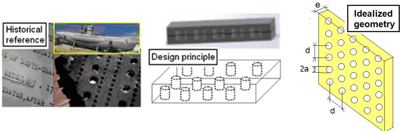
Figure 1: Principle of the Alberich-type acoustic coating, and geometrical parameters used in this study
